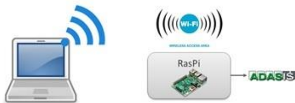
Figure 6: Wi-Fi connection between computer and Raspberry Pi
