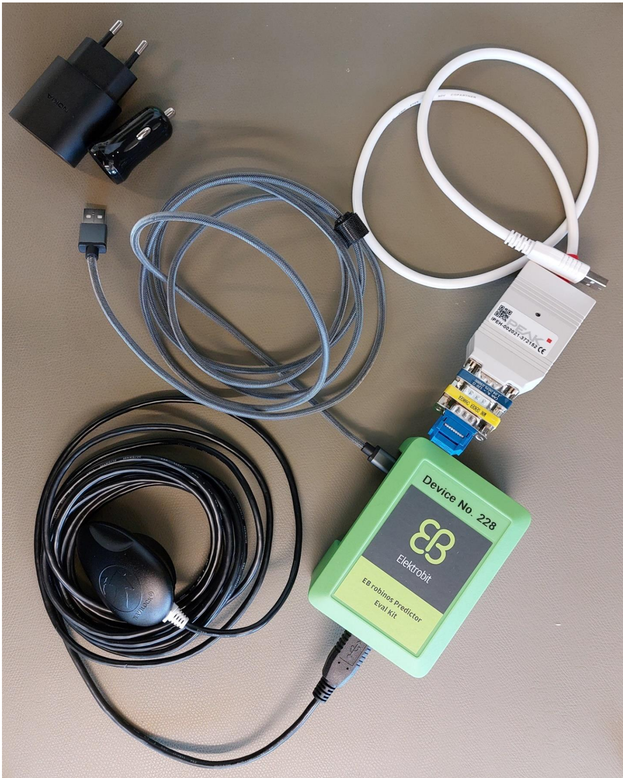
Figure 4: EB robinos Predictor Eval Kit with peripherals ready for use
