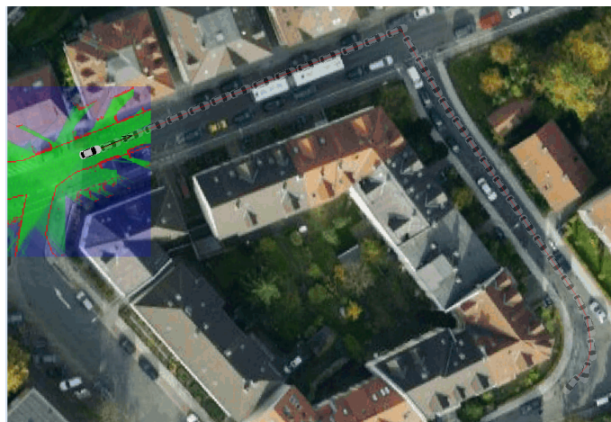
Figure 6.15. Screenshot of the EB robinos Path Planning visualization
