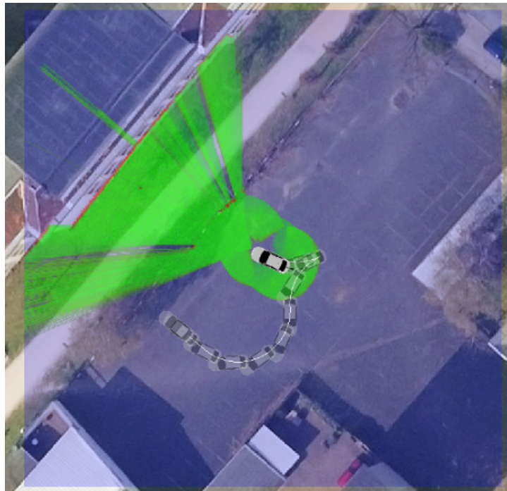
Figure 6.23. Screenshot of valet parking scenario while reversing
