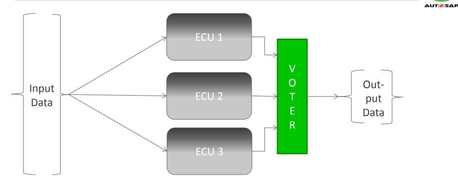
Three redundant ECUs calculate on redundant data, output data is voted upon
