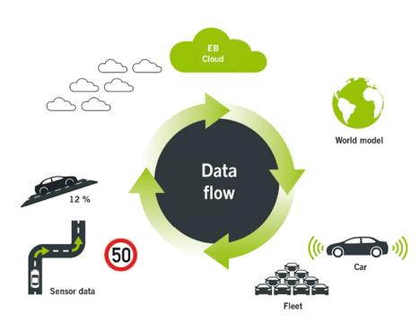
**FIGURE 1** Many vehicles have sensors that record data on speed, incline, curves and other information that is stored in the cloud, this information is used to supplement map material, thereby providing a more comprehensive picture of the worldwide road network
