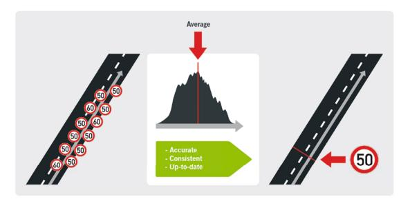
FIGURE 3 Several vehicles record and transfer data to the cloud about a specific road sign; these data records which vary in terms of exact location and perceived maximum speed limit, are then analysed by data mining; the objective is to update or verify existing sign information and to possibly include new road signs in the map material
