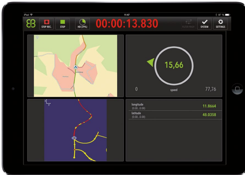
Clear representation of the electronic horizon, the map view and the vehicle data on an iPad
