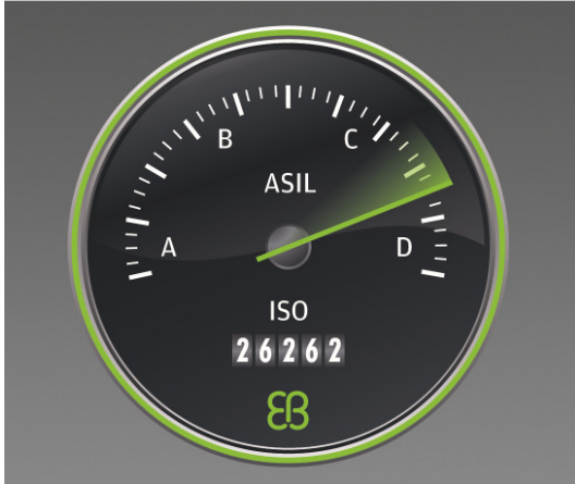
Fig. 4. Automotive Safety Integrity Level (ASIL) rates the safety relevance of errors on a scale from A to D according to the three criteria of driving situation frequency of occurrence, controllability of a situation when a function error occurs and severity of the consequences.
